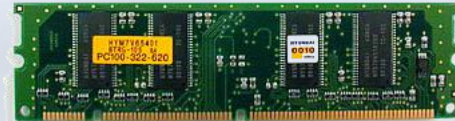
DIMM (Dual in-line memory module)
