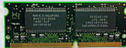
SODIMM (Small outline dual in-line memory module)
