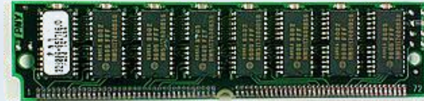
SIMM (Single in-line memory module)
