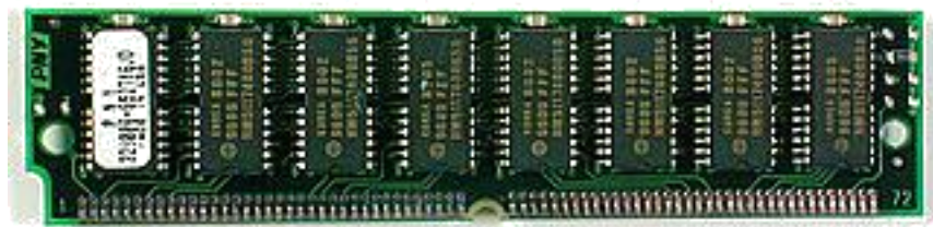
SIMM (Single in-line memory module)
